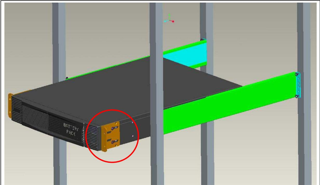
6. Slide the Battery Pack into position and using the screws to fasten the Brackets to the Front Posts of The Rack.
