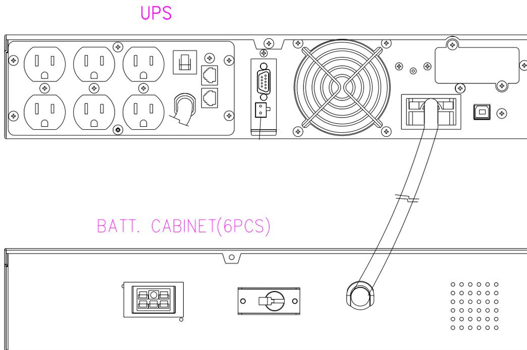
**Rear Panel View of 700VA ~ 1500VA UPS and EBP (12 pcs Batteries):**
