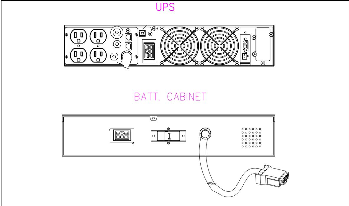
10. **Connect the Electrical Connections between UPS and Battery Pack.**
